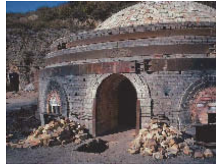
One of the many round, or down draught beehive bauxite kilns of Shanxi province which have faced enforced government closure for environmental reasons. The impact of which has been a shortage in supply of certain calcined bauxite grades.
